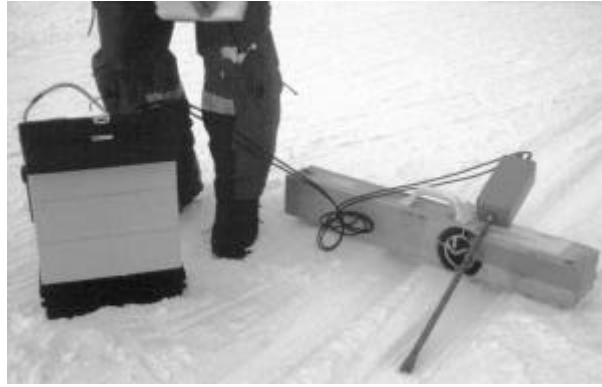
Fig. 5.2. Setup for snow surface measurements with the Snow Fork .
